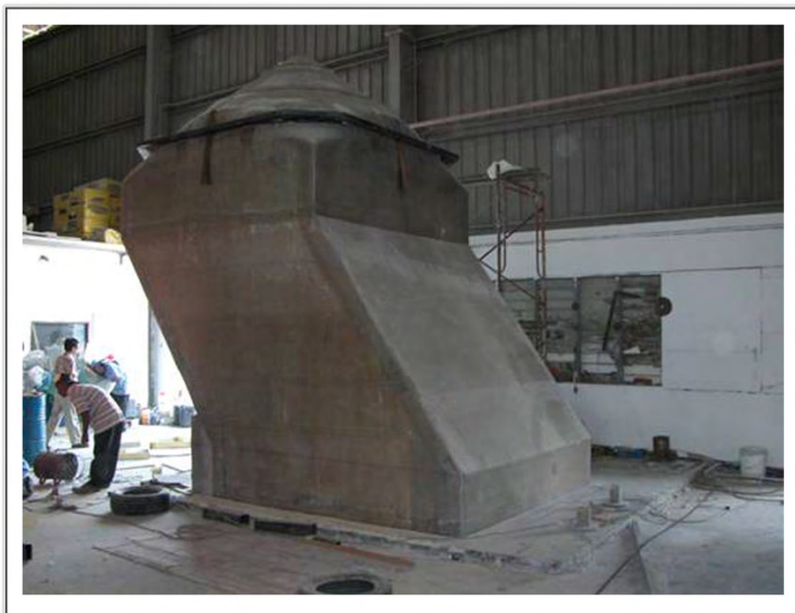
Clarifier Body Fabricaton
