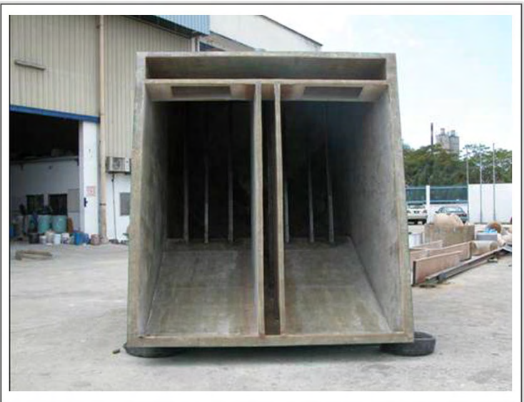
Plates Support @ Internal Clarifier
