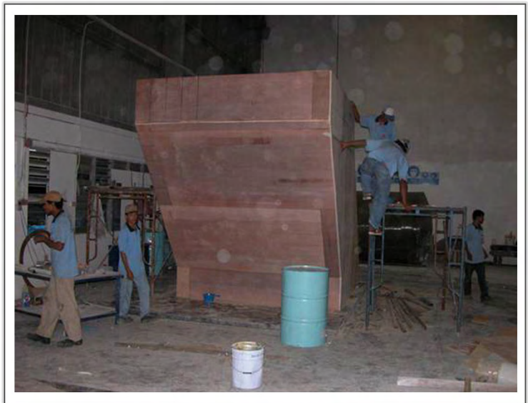
Mould Fabrication
